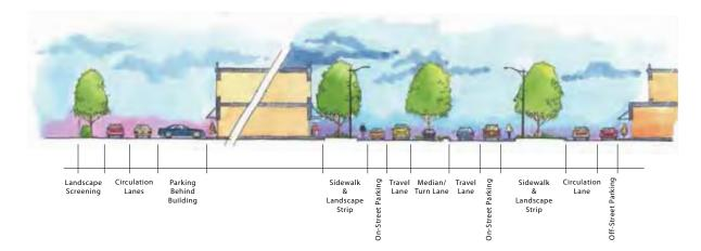
*Figure 4-24: Mid Block Residential Sub-Area/Roadway Cross Section*
