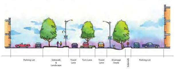
Figure 4-23: Age Restricted Sub-Area/Roadway Cross Section
